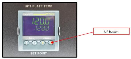
Figure 1 – Temperature display
