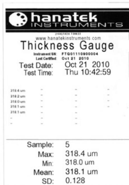
**Measurement tip- To include details of all measured results in the print out click the "Print All Results" option in the instrument set up menu.**
