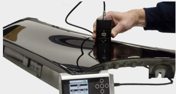
The Rhopoint IQ Flex 20 quantifies surface quality problems such as orange peel and haze that are invisible to a standard glossmeter. It profiles how light is reflected from a surface.
