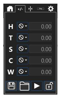
Pass/Fail tolerancing can be set for each/any of the metrics displayed. disabled.
