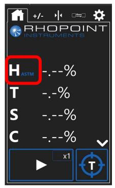
ASTM will be displayed after the H metric on the screen indicating that measurements comply to ASTM D1003.
