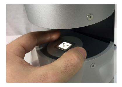
For fast easy manipulation high clarity samples with limited distance dependency, the user may manually hold and move the sample.
