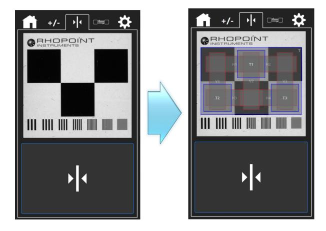
The alignment tab allows the user to see a live view of the graticule to aid in alignment of samples. It also allows the user to align the ROIS of the instrument automatically if the sample used is causing a linear optical offset.
