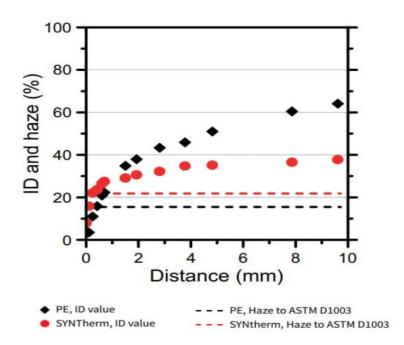
To match an end use application the distance between the sample and platen should match a chosen value based on those in the real-world application.
