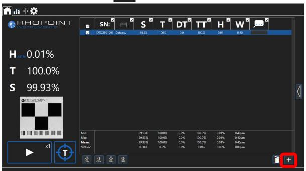
This will bring up the expanded table window for use with multiple screens and the ability to add hidden columns back to the main table.
