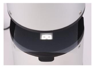
Measuring with the ASTM haze spacer in place is often the default method for most applications.
