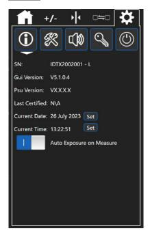
The settings tab provides system configuration and Power Off.
