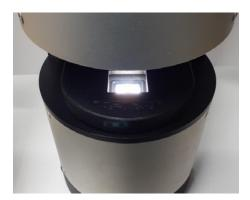
The standard locates in place by magnets; ensure that the standard can locate properly.
