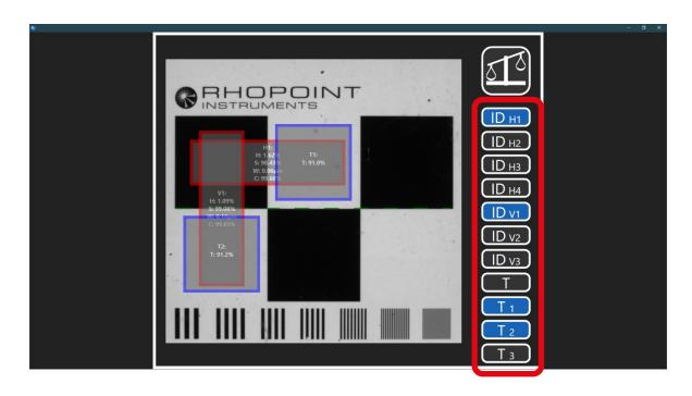
The on-instrument T value are calculated using the transmitted light through all black and white areas, this area can be viewed by toggling the T button.
