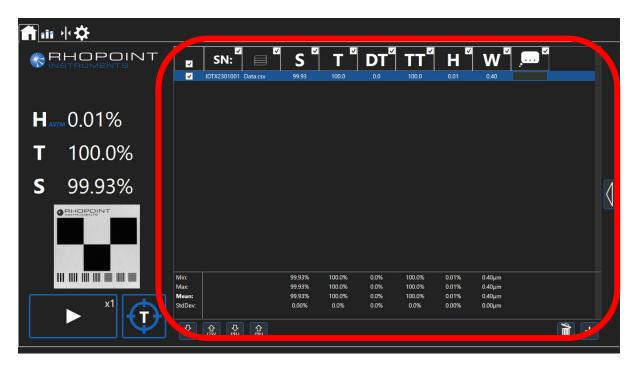
The center Panel of the software contains the results for all measurements taken in the current batch. The bottom section contains statistics for all the results listed in the table.
