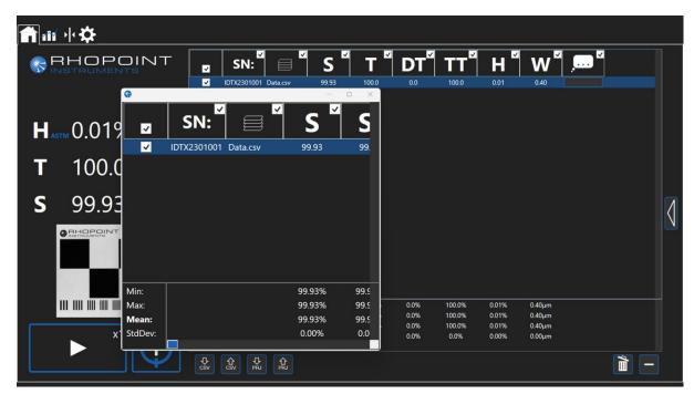
Clicking on the tick box in the top corner of any parameter will include/exclude it from the **ID Results Table.** Parameters can be dragged and dropped to rearrange columns as required and results can be copied to the clipboard by pressing Ctrl + C. This is available in both tables
