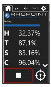
The instrument introduces a delay before starting the first measurement and between readings - this allows the user time to manipulate the sample. To finish any batch early press the stop button.
