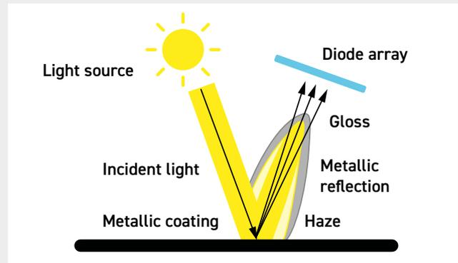
The IQ Flex 20-S captures compensation information from a region adjacent to the haze measurement angle. This means it can be used on metallic coatings which reflect light.
