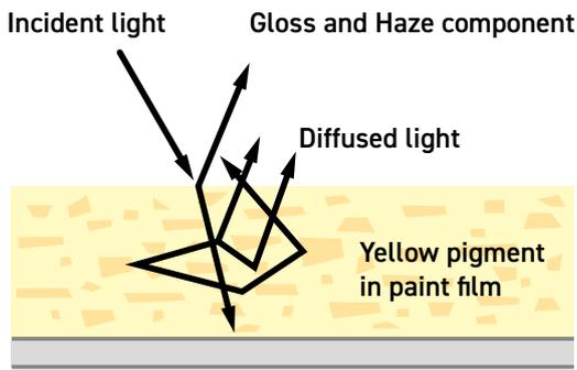
The IQ Flex 20-S compensates for reflection from within the coating for highly reflective pigments, metallic coatings and speciality pigments, allowing the haze of any painted surface to be measured.
