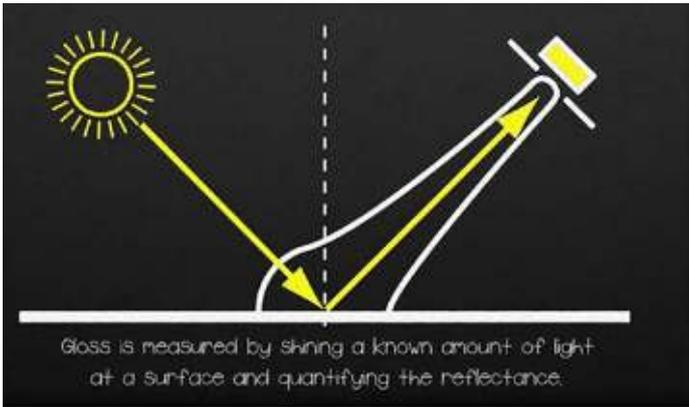
The angle of the light and the method by which the reflectance is measured are determined by the surface material and which aspect of the surface appearance is to be measured.
