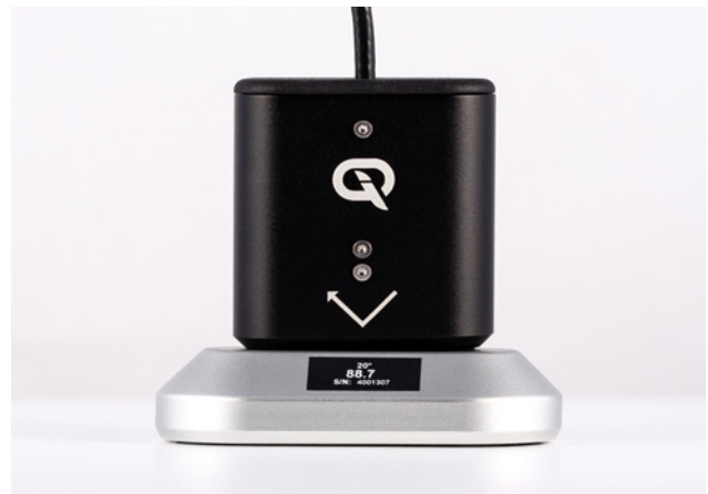
IQ Flex 20 with calibration tile
