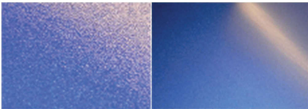
Example test panels with low and high DOI values. Orange peel, texture, flow out and other key parameters can be assessed in coating applications where high gloss quality is becoming increasingly important.
