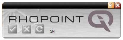
4. The buttons are greyed out while the DATA widget searches for SWITCHED ON IQ(s) that have been PAIRED to the PC.
