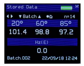
When Memory is set to ON (as detailed later in the Menu Screen section of this manual) measurements can be recalled and displayed from any batch stored in the IQ memory.
