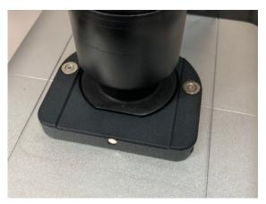
Take a reading on the checking standard by pressing the tick icon and compare the result with its assigned value. The value must match the assigned value within the tolerances printed on the label.
