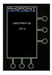
Once lamp warm up is complete the main measuring screen will be displayed. The tare icon will flash indicating an essential operation. Lower the light baffle then press and hold the tare button until a repetitive beep is heard. The unit will operate and set the zero reference.
