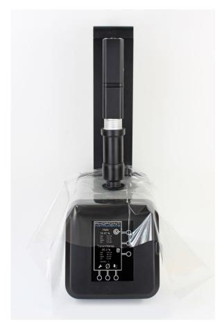
To take a reading, press the tick button. The instrument will operate and the results will be displayed on the screen. If a record of each reading is required, press the export button to send the result to a data stick or printer. See the export section of this manual for more details. Continue taking readings by pressing the tick button. Statistics are updated with each measurement. To reset the statistics delete the readings from the instrument memory (see below).
