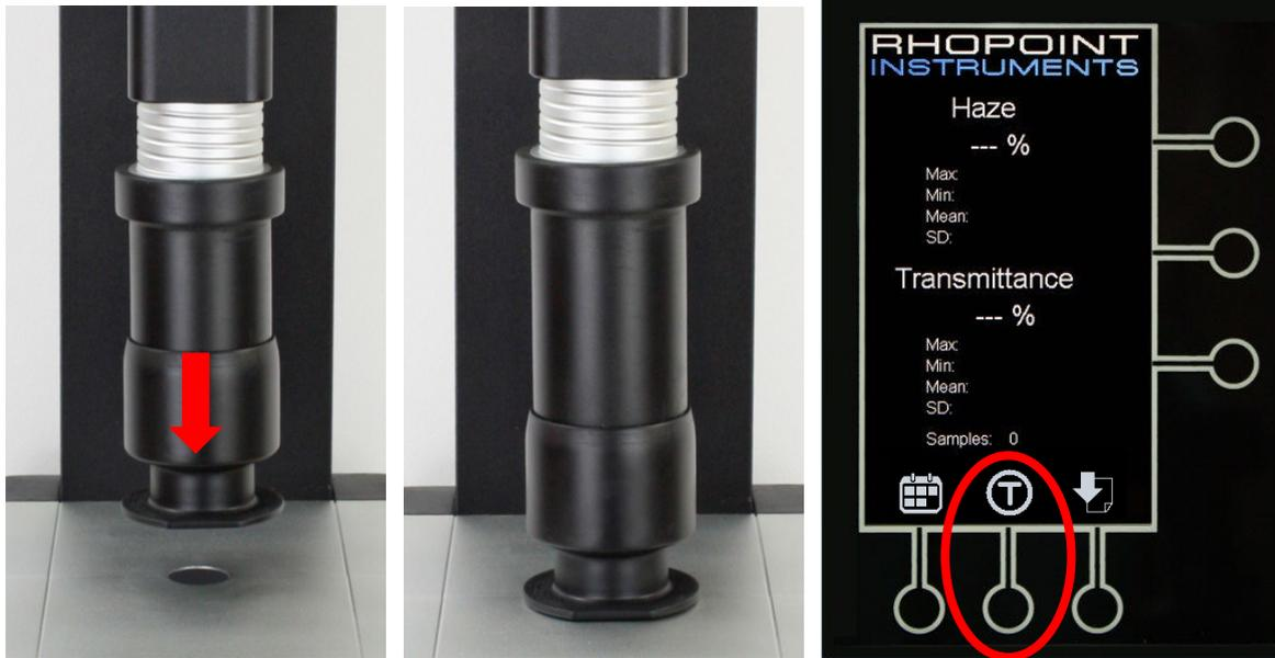
The measuring icon (tick) will now be displayed on the screen (see below). The instrument is now ready to take readings.
